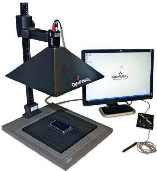
Figure 1. Complete WatchDog test set up for mobile device testing
