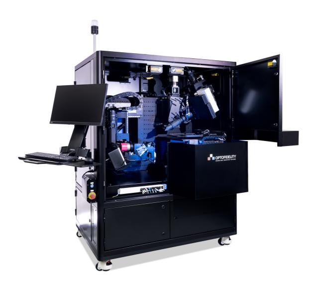
Fully automated waveguide image quality measurement system
