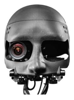
Measure motion-to-photon latency, content stability and pose-drifting with BUDDY, which is suitable for both AR and VR glasses.
